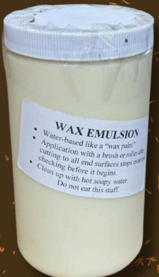
Always seal the ends of the boards, after cutting them. It Prevents ends from checking
